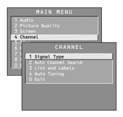
**Auto Channel Search** Tells the TV to search automatically for all the channels available through the antenna input. When the TV finds an active channel, it places it in the channel list; inactive channels (weak stations or channels with no signal at all) will be removed from the channel list. If you are using a cable box and have setup your GUIDE Plus+ system, this option will not appear.
